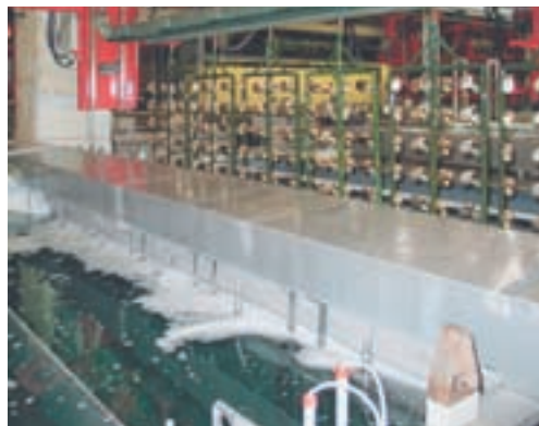
Rinsing tank with ultrasonic cleaning on both sides for optimal performance
