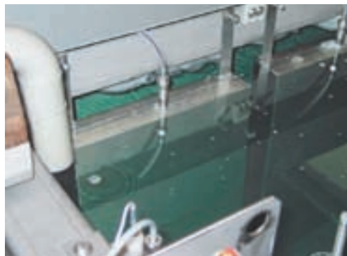
Specially alloyed and wired encapsulated transducer in operation in the electroplating unit
